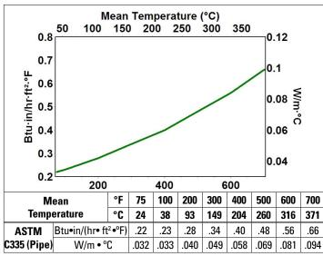
\*MinWool-1200 Pipe Insulation is tested in accordance with ASTM C335.
