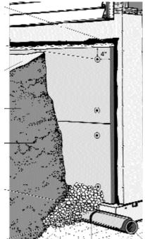
•DrainBoard must be installed over code approved dampproofing material.
